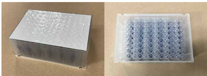
Figure 1. A sealed KingFisher 96 Deep-Well Plate. After filling wells in alternating rows of the plate with dyed liquid, the plate was sealed with Easy-Peel foil laminate using the ALPS5000 Automated Plate Heat Sealer and inspected for leaks.
