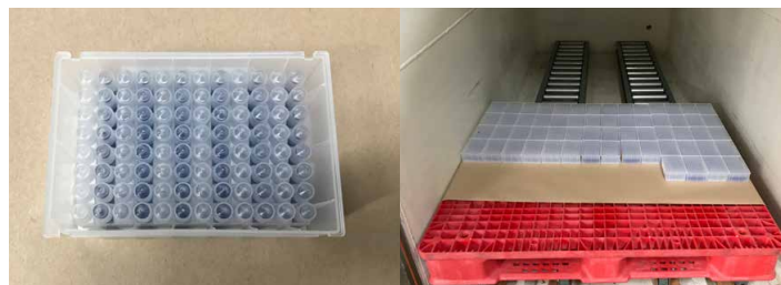
Figure 2. KingFisher 96 Deep-Well Plate inverted on absorbent material for leak inspection prior to testing (left) and the vacuum chamber in which sealed plates were subjected to low-pressure testing (right).
