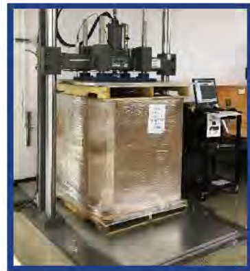
Figure 3 – Pallet Compression Test
