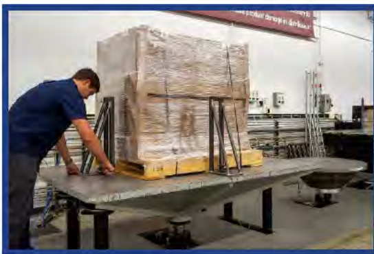
Figure 2 – Setting Up a Vibration Test
